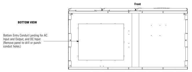
Figure 4-18. ISBM Section Conduit and Wire Entry Locations
